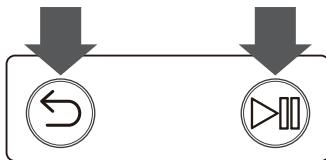
When you turn on the TV for the first time, the Samsung Smart Remote pairs to the TV automatically. If the Samsung Smart Remote does not pair to the TV automatically, point it at the remote control sensor of the TV, and then press and hold the buttons labelled and as shown in the figure on the left simultaneously for 3 seconds or more.
