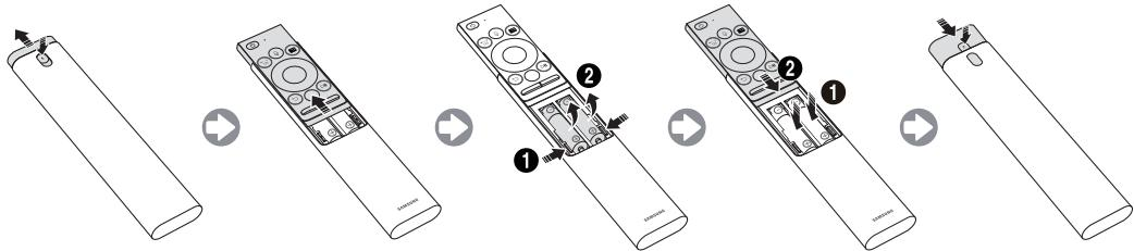
1. Press the at the top rear of the Samsung Smart Remote. The body will pop out slightly from the body cover.
